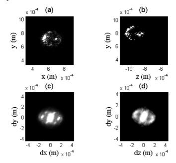
Fig. 4 In-focus images of a freezing droplet observed with (a) sensor 1 and (b) sensor 3; two-dimensional autocorrelations of the in-focus freezing droplet observed (c) in (a) and (d) in (b).
