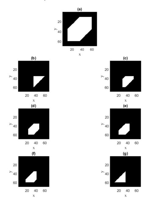
Fig. 7 2D-autocorrelation of an initial 2D-shape (a), and 6 possible 2D-objects whose 2D-autocorrelation is the one of Fig. (a) (b-g) (units in pixels); corresponding to a first angle of view.
