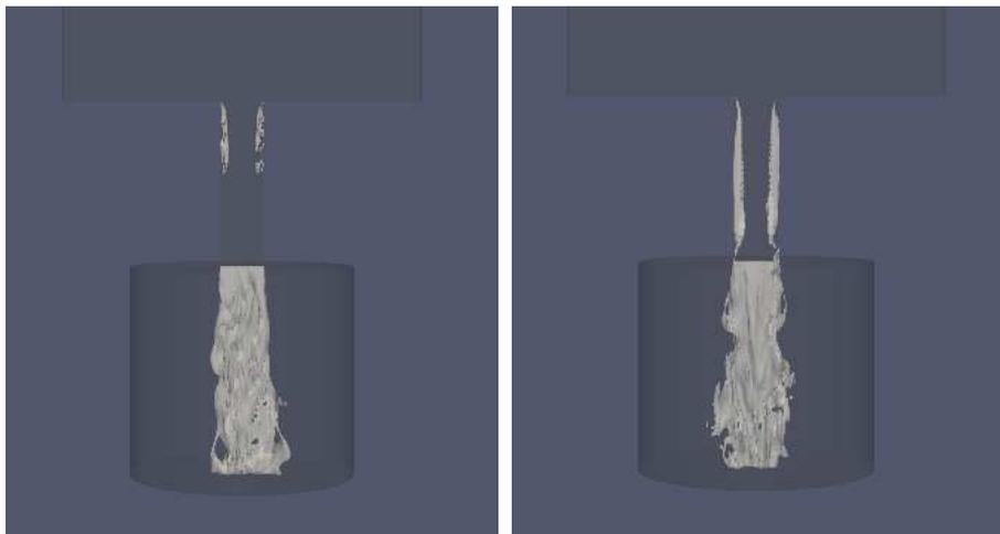
**Figure 1.** Simulations of the Sou's experiments. Cavitation number of 0.94 (left) and 0.65 (right)
