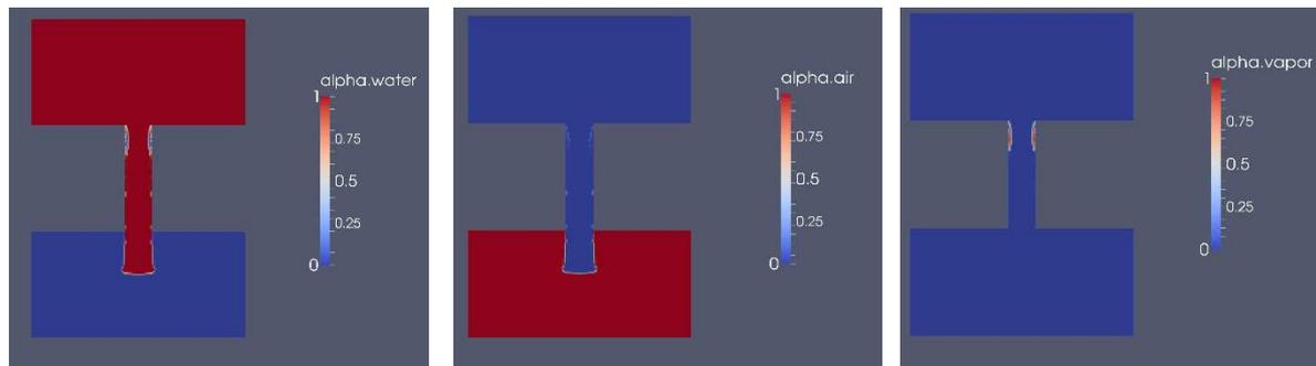
**Figure 2.** Simulation of cavitating injection: liquid, vapour and air volume fraction fields
