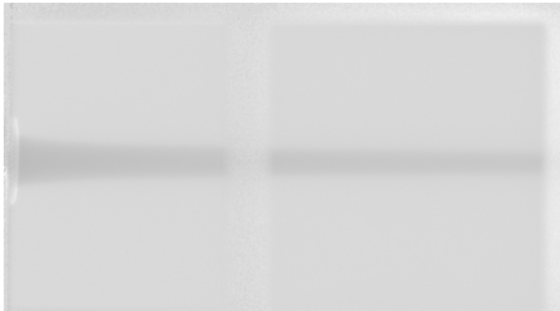
Figure 7: Radiography (22 mm long) of a jet of Ethane into Helium at 5.5 MPa and T_{ch} = 293 K. V_{inj} = 0.27 m.s -1 .
