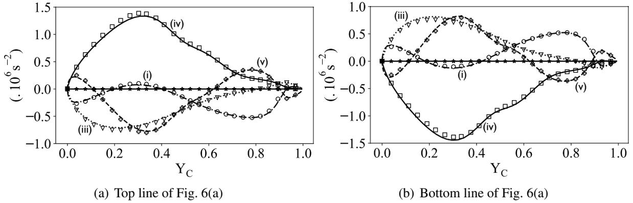
Figure 7: Vorticity budget versus  $Y_{CO_2}/Y_{CO_2}^b$  along the dashed-lines of Fig. 6. Lines: With gravity. Symbols: Without gravity. Circles: (i) of Eq. 3. Triangles: (iii). Squares: (iv) Baroclinic torque. Crosses: (v). Stars: budget.
