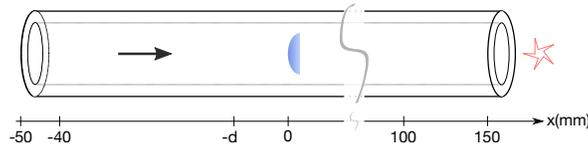
Figure 1: Schematic view of the experimental set-up composed of a quartz tube of  $\ell_i = 5$  mm inner diameter and  $e_w = 1$  mm thickness, inside which a lean methane/air mixture is injected. The inlet ( $x_i = -50$  mm) is connected to the mass flow controllers while the outlet ( $x_e = 150$  mm) is in open-air, where the flame is first ignited to then propagate inside the tube.
