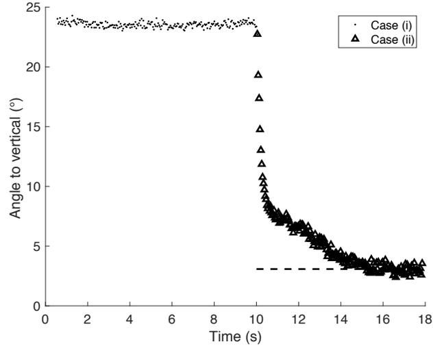
Figure 5: Time evolution of the flame angle to the vertical.  $t = 0$  denotes the decrease in mass flow rate. Dotted: Stabilised flame with heat-conductive wall (case (i)). Triangle: Propagating flame with iso-thermal wall (case (ii)).
