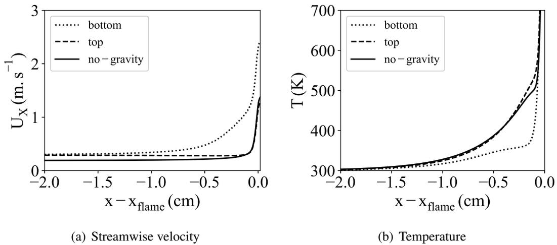
Figure 3: Streamwise velocity and temperature distribution at a distance of 0.7 mm from the top and bottom walls.  $x_{\text{flame}}$ : maximum of heat release on the probed line (top or bottom). No-gravity: symmetrical flame.
