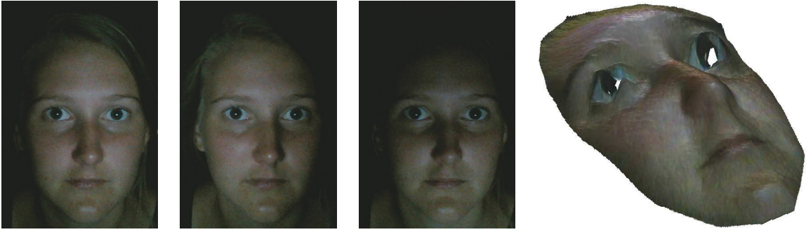
Figure 4. 3D-reconstruction using PS with extended anisotropic light sources. Left: 3 of the m = 4 input images, obtained by displaying white rectangular patterns on the screen of a laptop, and capturing the images using the laptop's integrated webcam. Right: 3D-reconstruction (the eyes were manually removed from the reconstruction domain). In this experiment, we used the RGB values instead of the graylevels, which allowed us to recover RGB albedos, as explained in Ref. 13.
