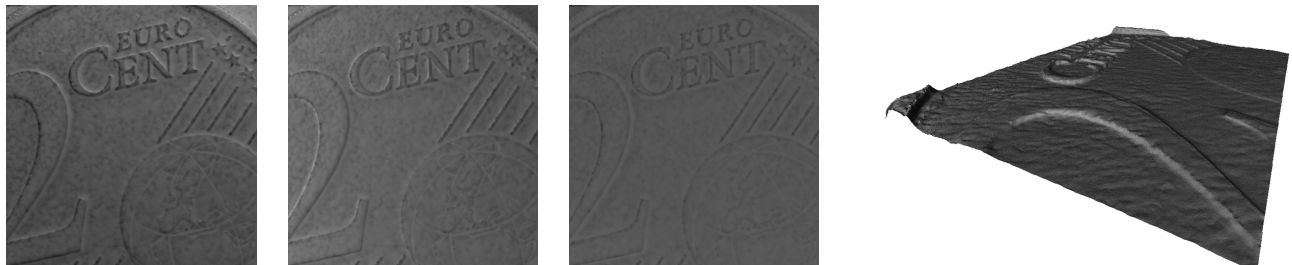
Figure 5. 3D-reconstruction using PS with complex primary lightings. Left: 3 of the m = 15 input images. In each image, the scene is illuminated by a combination of primary and secondary illuminants (LEDs and their reflections inside the device), which is sampled by introducing a planar calibration grid, before interpolation. Right: 3D-reconstruction. Both high- and low-frequency details are finely recovered.
