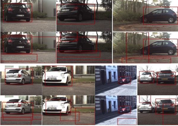
Fig. 5. Detection results. The first and third rows refer to the polar-based model whereas the second and fourth rows are the corresponding color-only based model.
