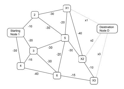
Fig. 1: Example of Maritime Shipping Graph with 3 variable edges (x1, x2, x3) to the destination D (dashed lines on the graph).{1,2,3,4,5,6} is the set S of stable nodes and {X1, X2, X3} is the set P of non stable nodes.
