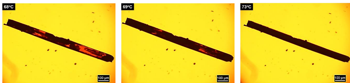
Figure 14. (a) Hot-stage microscopy (HSM) observation on the desolvation process of BDMC-ACET with increasing temperature at 5\text{ }^{\circ}\text{C}\cdot\text{min}^{-1} . Several nucleation sites of the non-solvated component are observed.
