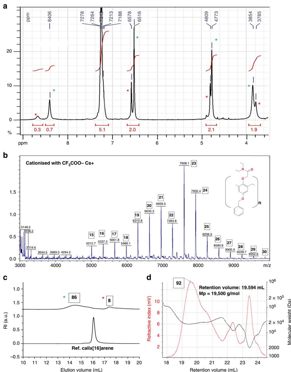
**Fig. 7** Analysis of a sample with a size range centered around 90 PRUs as the main specie. **a**  $^1\text{H}$  NMR (DMSO- $d_6$ ); **b** linear mode MALDI-TOF MS ( $\text{Cs}^+$  cationized); **c** SEC; and **d** SEC-MALS analyses of the largest calixarenes isolated (two-step process, 0.8 equivalent of  $\text{RbOH}$  vs phenol). PRU numbers are shown in boxes. The red and green asterisks are referring to calix[8]arene and giant calixarenes, respectively
