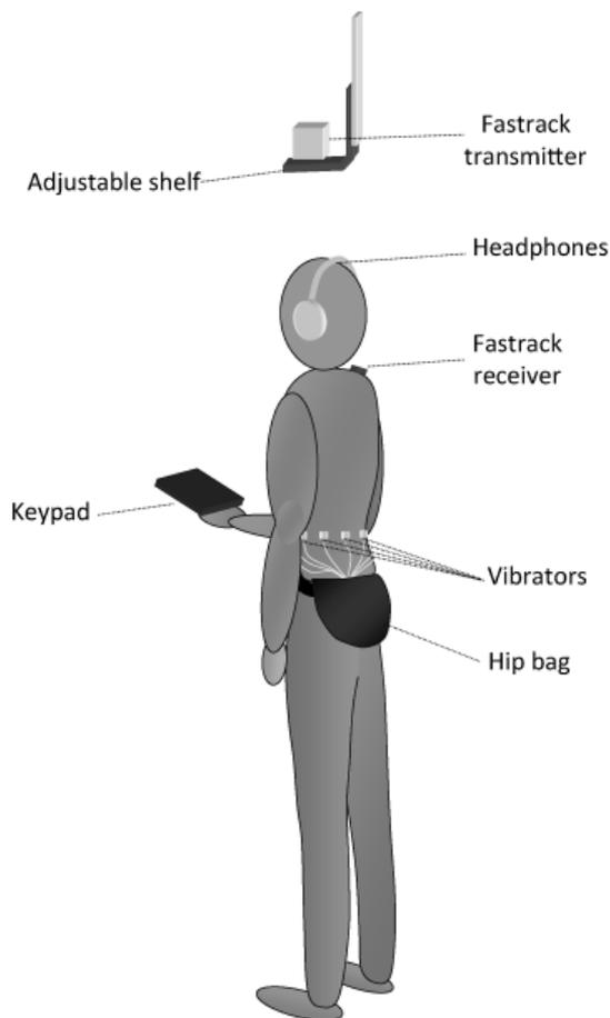
Figure 2. Schematic view of the experimental set-up.
