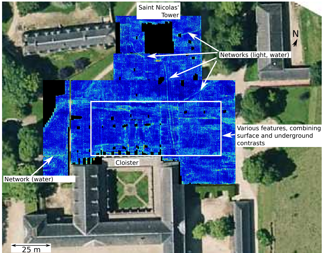
Figure 5: GPR slice at 0.3 m depth.
