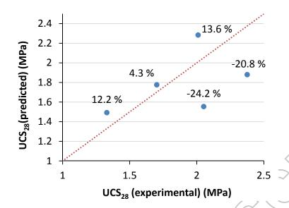
Figure 8. Validation of equation 6; UCS<sub>28</sub> (predicted) vs UCS<sub>28</sub> (experimental)
