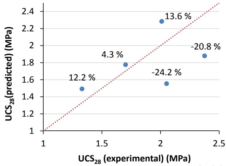
Figure 8. Validation of equation 6; UCS<sub>28</sub> (predicted) vs UCS<sub>28</sub> (experimental)
