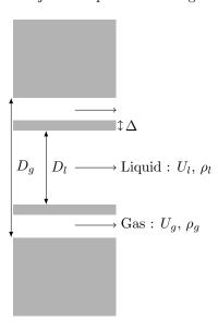
Figure 13: Schematic of the injector used by Stepowski et al. [37].
