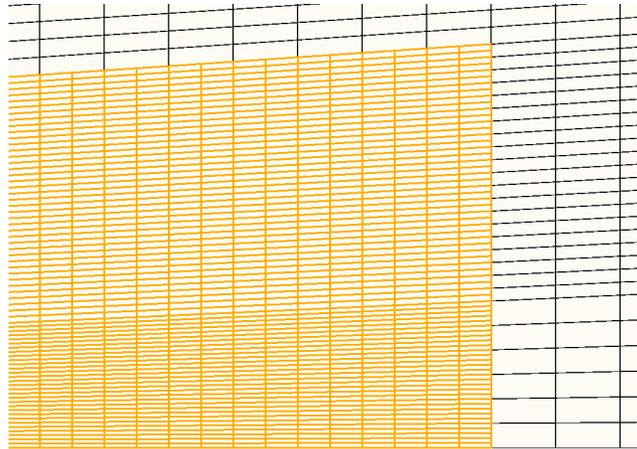
Figure 9: Zoom on the fine zonal mesh, shown in yellow. The fine mesh refinement relative to the coarse refinement is 5 : 1 in the y-direction close to the jet center line and 2 : 1 otherwise.
