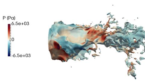
Figure 15: Three-dimensional snapshot of the phase indicator isosurface  $\alpha = 0.5$  obtained with the *fine zonal hybrid* simulation, along with the dynamic pressure field. The zonal interface  $\Gamma$  is shown with a black line.
