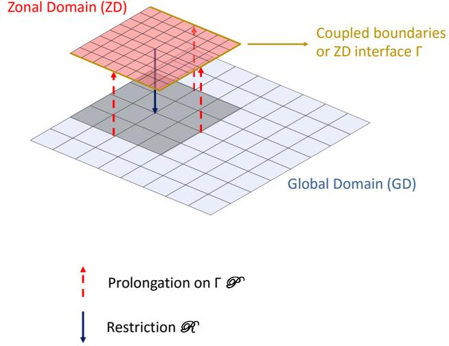
Figure 1: Global and zonal domains. Global domain (GD) is the main computational domain while Zonal Domain (ZD) is fully overlapped in GD. Communication from GD to interface  $\Gamma$  is done via the prolongation  $\mathcal{P}$  operator. Communication from the ZD field to the underlying GD field is done via the restriction  $\mathcal{R}$  operator.
