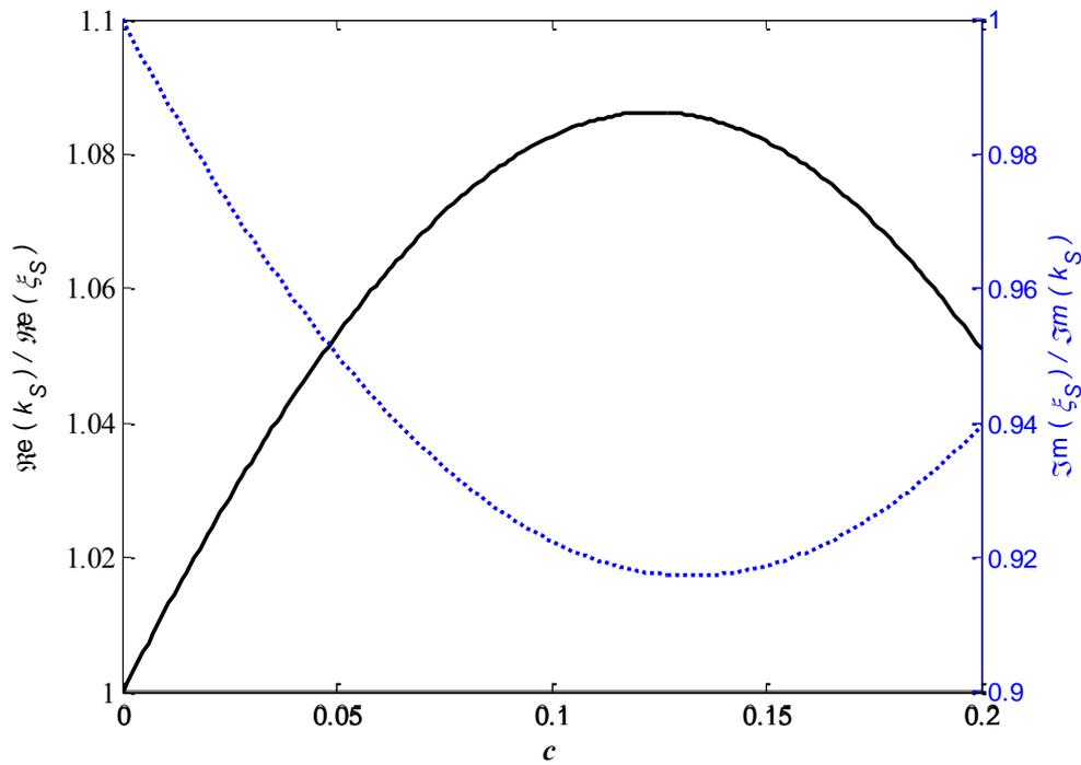
**Figure 4.** Ratios of the effective shear wave velocity (solid line, left vertical axis) and attenuation (dotted line, right vertical axis) to those of the shear wave in the absence of scatterers, versus concentration.
