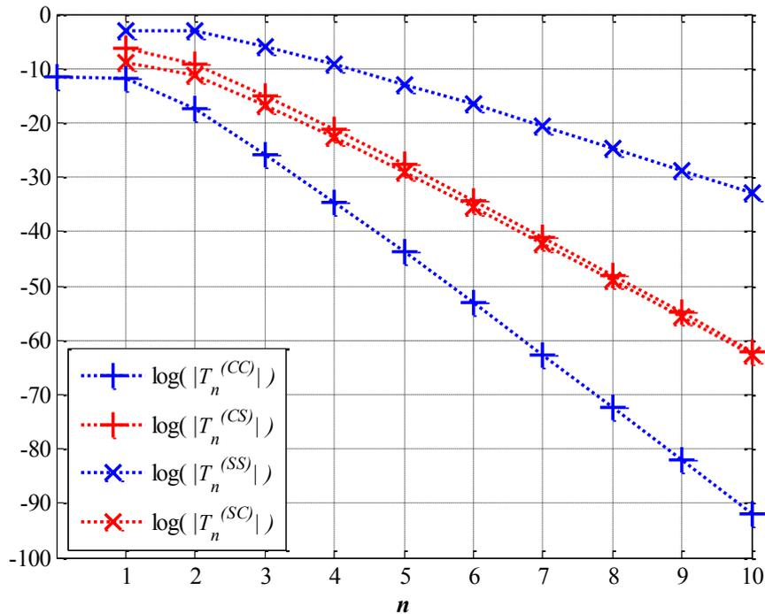
**Figure 1.** The modal scattering coefficients (amplitudes) as functions of mode number.
