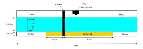
Fig. 1. Sketch of the experimental setup
