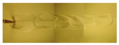
Fig. 3. Sedimentary structures downstream the cylinder; Re=38000 (Test 1)
