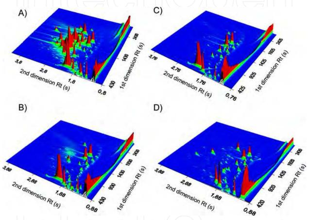
Fig. 6. 3D contour plots of four rivers sampled in this study in which the total ion chromatogram is shown: Ebro (A), Llobregat (B), Ter (C), and Beso`s (D). Reprinted with permission from Analytical Chemistry, (Matamoros et al., 2010a). Copyright 2011 American Chemical Society.
