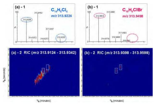
Fig. 3. The difference of isotope patterns between two peaks in the soil extract; (a)-1  $C_{14}H_6Cl_4$  and (b)-1  $C_{16}H_8ClBr$  and GC×GC-HR TOFMS 2D exact mass chromatogram of a 0.02 Da wide windows (a)-2  $C_{14}H_6Cl_4$ ; m/z 337.9224 and (b)-2  $C_{16}H_8ClBr$ ; m/z 313.9498. Reprinted from Publication, Journal of Chromatography, A, (Ieda et al., 2011). Copyright (2011), with permission from Elsevier.
