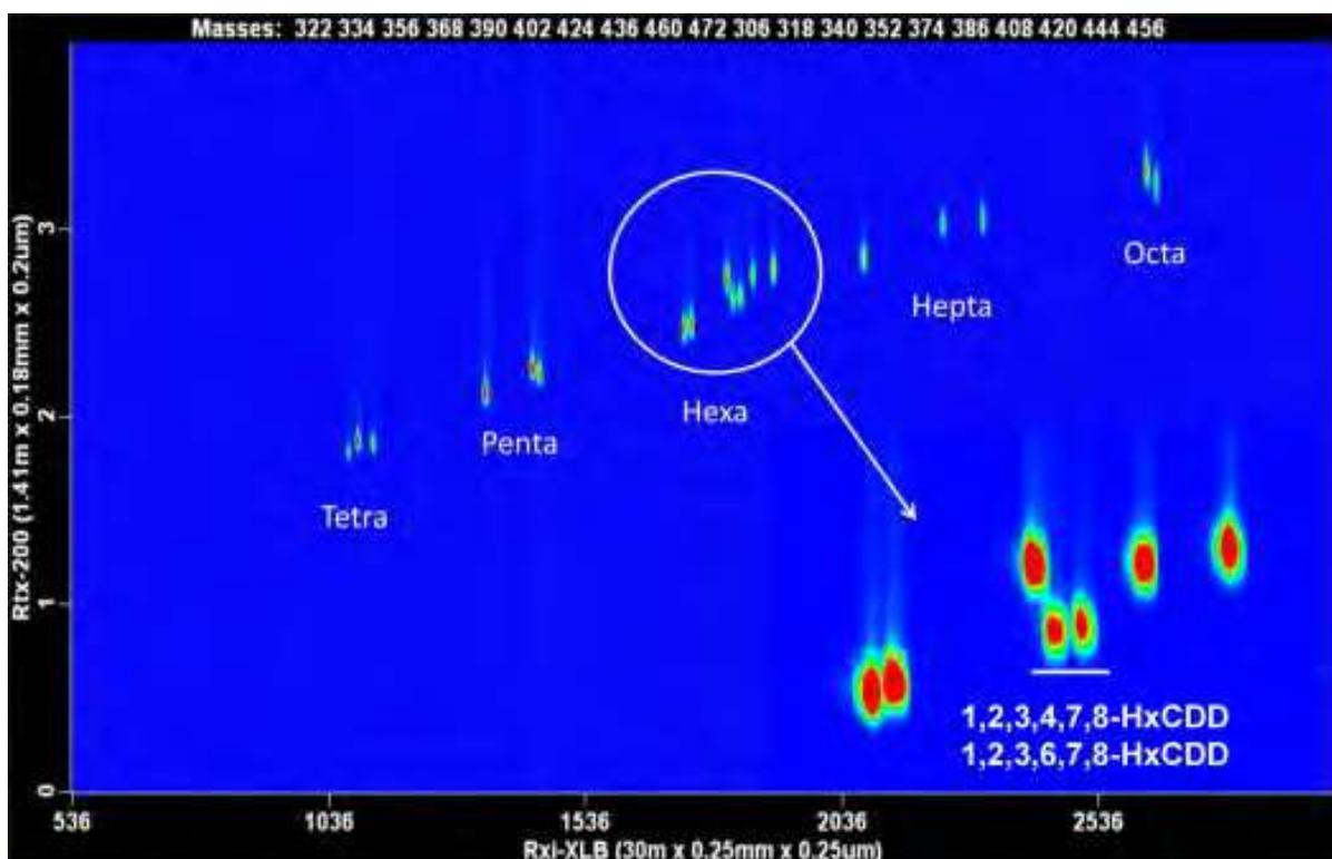
Fig. 2. <sup>2</sup>D selected ion contour plot for the 17 priority PCDD/Fs using the Rxi-XLB/Rtx-200 column combination. The PCDD/Fs are again well resolved, especially the 1,2,3,4,7,8-HxCDD and 1,2,3,6,7,8-HxCDD isomers. Reprinted from *Journal of Chromatography, A*, (de Vos, 2011a). Copyright (2011), with permission from Elsevier.
