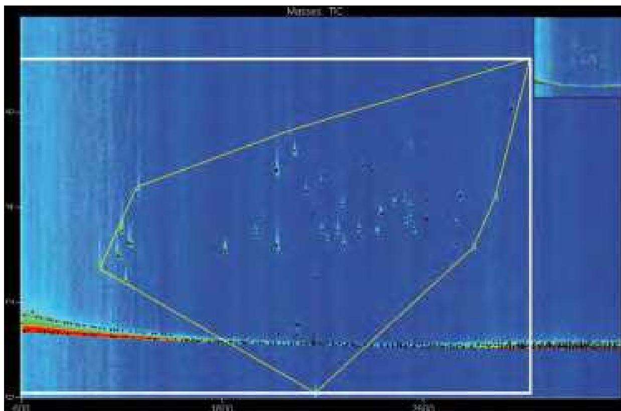
Fig. 9. Chromatogram illustrating the retention space used (white) and the space used calculated with Delaunay's triangulation algorithms (yellow) obtained on HP5-Mega225. Reprinted from *Journal of Chromatography, A*, (Semard *et al.*, 2010). Copyright (2010), with permission from Elsevier.
