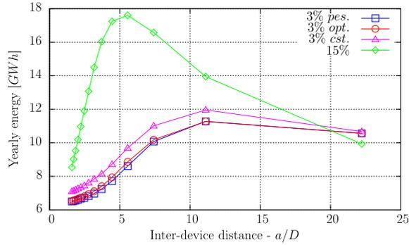
**Fig. 7.** Evolution of the yearly energy production in *GWh* with the number of installed turbines and presented with respect to inter-device distances. Comparison between the 3% and 15% of ambient turbulence. For the 3% ambient turbulence case, the three scenarios of Section 3.2 are analysed regarding the  $C_p$  evaluation.
