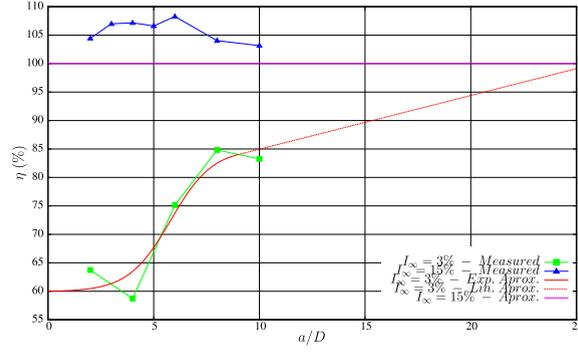
**Fig. 2.** Efficiency of the downstream turbine function of the dimensionless inter-device distance  $a/D$  depending on the ambient turbulence intensity  $I_\infty$ . Data are reproduced from Ref. [31].
