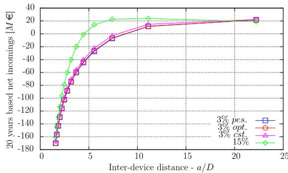
**Fig. 8.** Evolution of 20 years based net incomings in *M€* with the number of installed turbines and presented with respect to inter-device distances. Comparison between the 3% and 15% of ambient turbulence. For the 3% ambient turbulence case, the three scenarios of Section 3.2 are analysed regarding the  $C_p$  evaluation.
