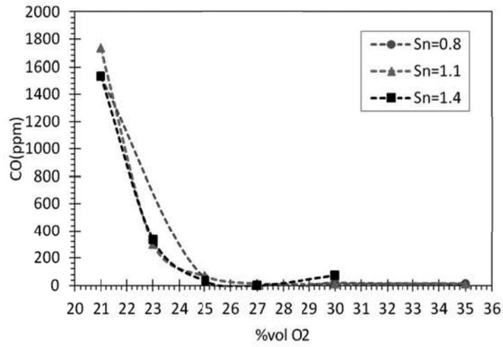
**Figure 17.** CO emissions with O<sub>2</sub> enrichment at  $\phi = 1$  for three swirl numbers 0.8, 1.1 and 1.4.
