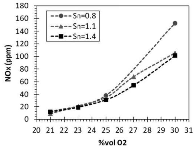
**Figure 11.** NO<sub>x</sub> emissions with O<sub>2</sub> enrichment at  $\phi=1$  for three swirl numbers 0.8, 1.1 and 1.4.
