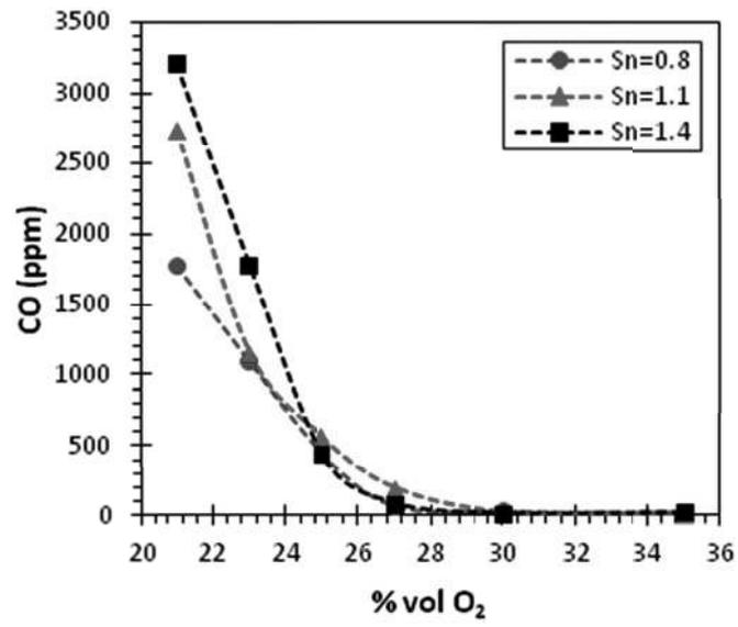
**Figure 14.** CO emissions with O<sub>2</sub> enrichment at  $\phi = 0.8$  for three swirl numbers 0.8, 1.1 and 1.4.
