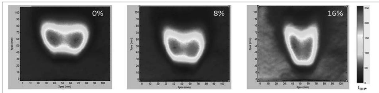
**Figure 8.** Average images of OH\* chemiluminescence without CO<sub>2</sub> dilution (0% of CO<sub>2</sub>) and with CO<sub>2</sub> dilution (8 and 16%) for Sn = 1.4 and  $\phi = 0.8$ .
