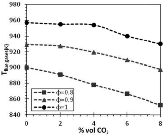
**Figure 13.** Temperatures of flue gases with O<sub>2</sub> enrichment (left) and CO<sub>2</sub> dilution (right) for Sn=0.8 at three equivalence ratios  $\phi=0.8$ , 0.9 and 1.
