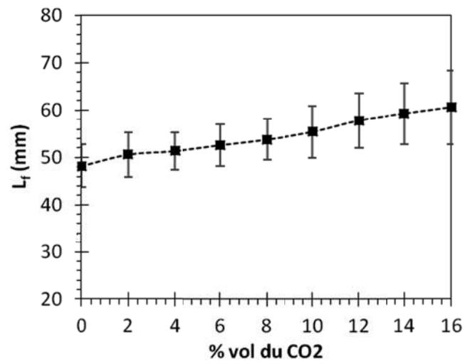
**Figure 10.** Flame length with CO<sub>2</sub> dilution for Sn = 1.4,  $\phi = 0.8$  and 21%vol of O<sub>2</sub> in the oxidizer.
