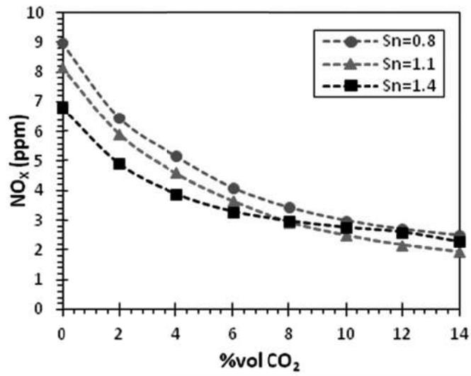
**Figure 12.** NO<sub>x</sub> emissions with CO<sub>2</sub> dilution at  $\phi = 0.8$  and 21%vol of O<sub>2</sub> for three swirl numbers 0.8, 1.1 and 1.4.
