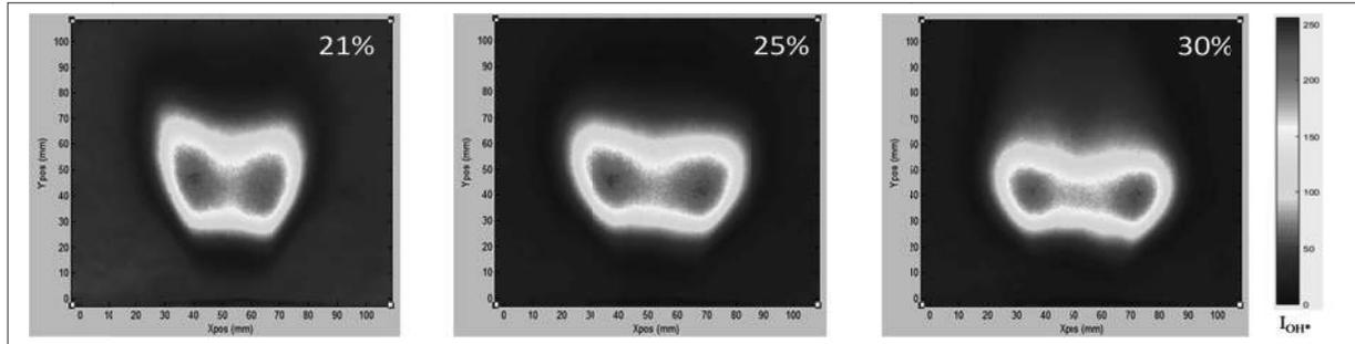
**Figure 5.** Average images of OH\* chemiluminescence without O<sub>2</sub> enrichment (21%) and with enrichment (25 and 30%) for Sn=1.4,  $\phi = 0.8$  and 10%vol of CO<sub>2</sub> in the oxidizer.
