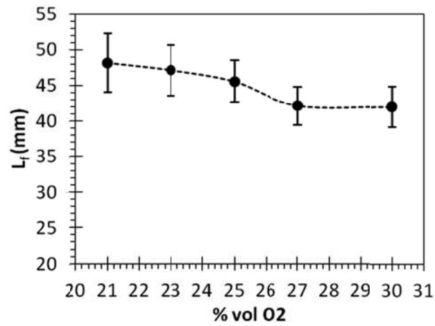
**Figure 7.** Flame length with oxygen enrichment for  $\phi = 0.8$ ,  $Sn = 1.4$  and 10 % vol of CO<sub>2</sub> in the oxidizer.
