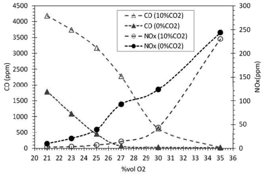
**Figure 18.** Combination of NOx and CO emissions with CO<sub>2</sub> dilution for 21 and 25% of O<sub>2</sub> enrichment, in the case of Sn=1.4 and  $\phi = 0.8$ .
