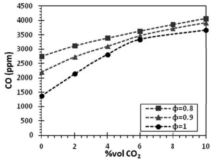
**Figure 15.** CO emissions with CO<sub>2</sub> dilution for Sn = 0.8 and 21%vol of O<sub>2</sub> at three different equivalence ratios  $\phi=0.8, 0.9$  and 1.
