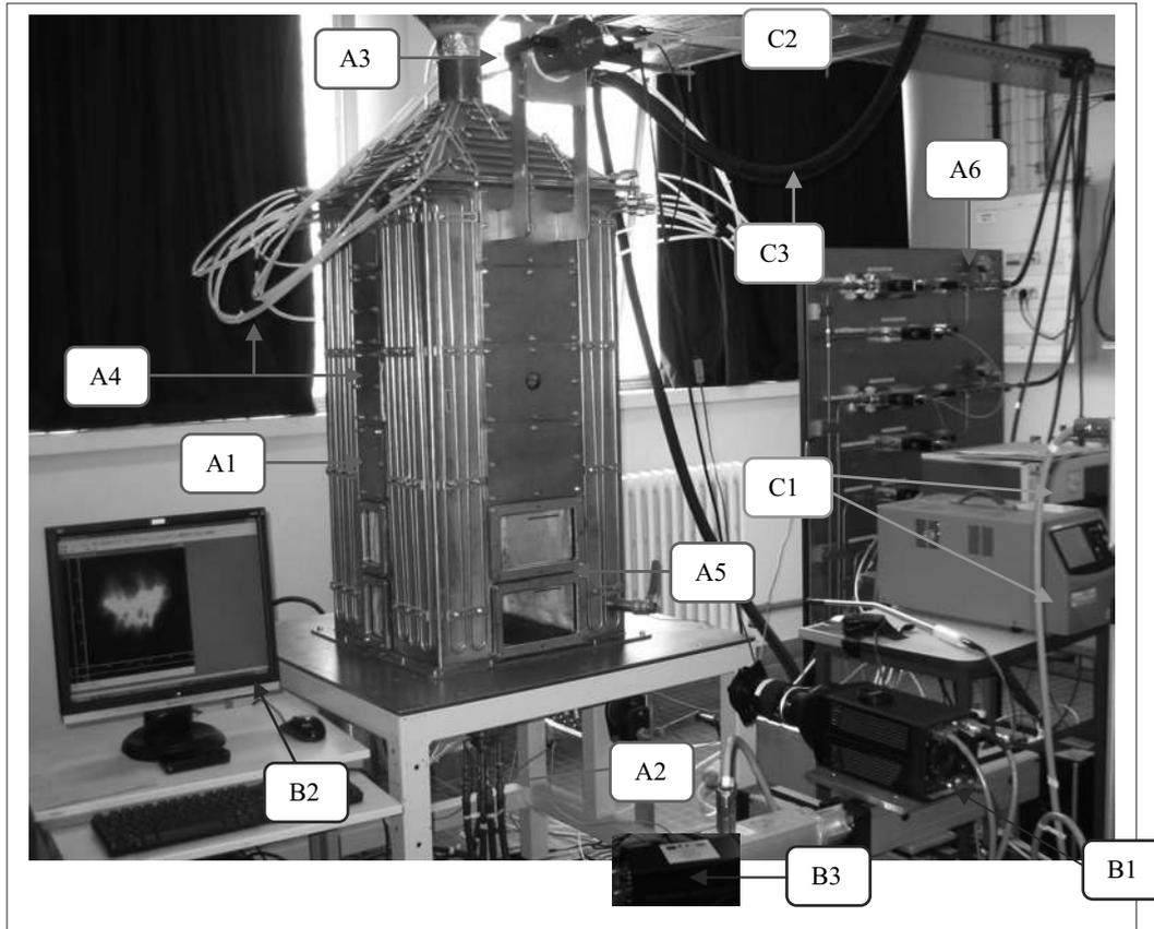
**Figure 1.** Experimental facility: combustion chamber (Ai, A1: combustion chamber, A2: coaxial burner, A3: extraction tube, A4: cooling water system, A5: windows of visualization, A6: gas supply panel), chemiluminescence system (Bi, B1: ICCD camera, B2: computer, B3: camera intensifier) and gas analyzers with sampling probe (Ci, C1: gas analysers, C2: sampling probe (PSP4000-HCT), C3: heated gas transport line).
