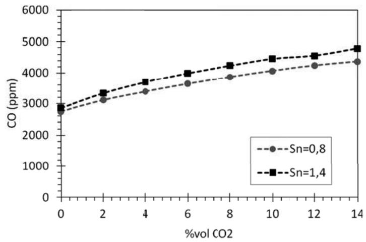
**Figure 16.** CO emissions with CO<sub>2</sub> dilution at  $\phi = 0.8$ , 21% of O<sub>2</sub>, and for Sn= 0.8 and 1.4.
