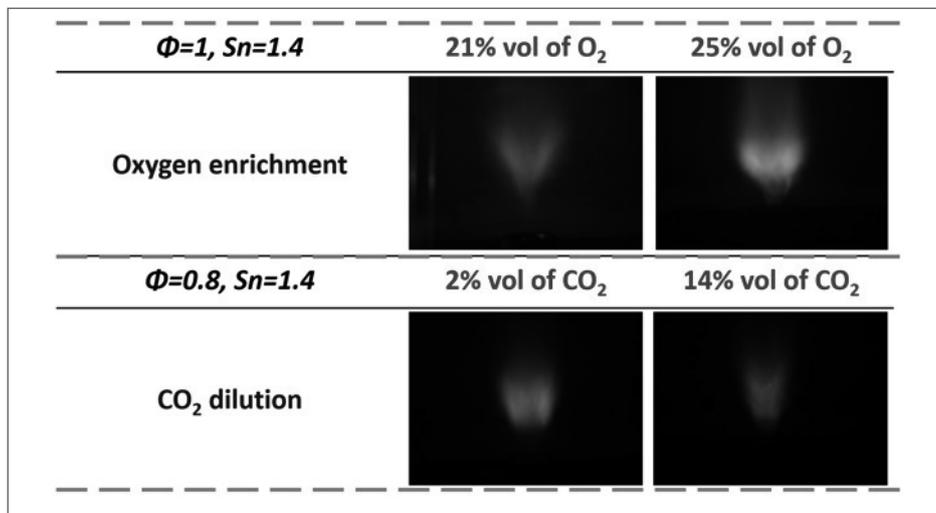
**Figure 3.** Examples of flame images with oxygen enrichment (top) and CO<sub>2</sub> dilution (bottom)
