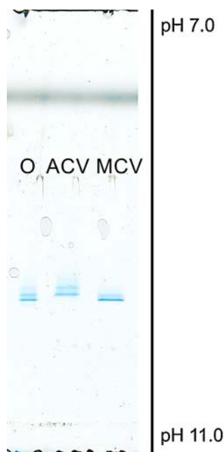
Fig. 4. IEF gel of the initial mAb (O), the acidic charge variants (ACV) and the main charge variant (MCV). A faint band is visible with a pI lower than the main band in the MCV standard. No main band can be detected in the ACV standard.
