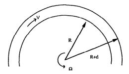
FIG. 1. Sketch of the flow geometry: flow between two fixed coaxial cylindrical surfaces under constant external pressure gradient. The rotation axis coincides with that of the system.
