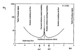
FIG. 2. Phase diagram ( $\tilde{R}o, De_c$ ): different regimes shown for  $\delta = 0.001$ .
