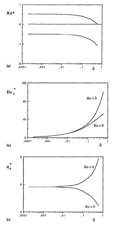
FIG. 3. Wide gap size effects on critical parameters at the restabilization point: (a)  $\tilde{Ro}^*(\delta)$ ; (b)  $De_c^*(\delta)$ ; (c)  $q_c^*(\delta)$ .
