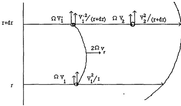
FIG. 4. Sketch for formulation of generalized inviscid Rayleigh discriminant using the displaced particle argument: shown are Coriolis and centrifugal accelerations of the particle at positions  $r$  and  $r + dr$ .
